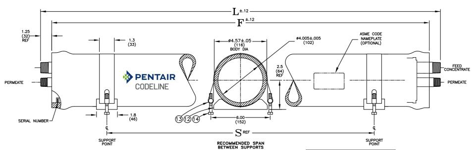
CENTER VESSEL ON 2 OR 3 SUPPORTS AT SPAN(S) "S" : 3 SUPPORTS REQUIRED FOR LENGTHS -4 AND OVER
